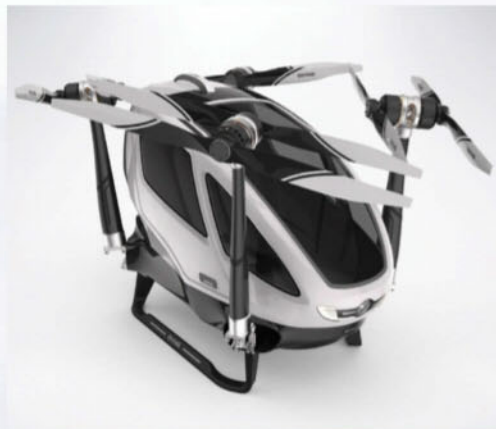
The drone is less than two metres tall, and the arms can be folded for storage
