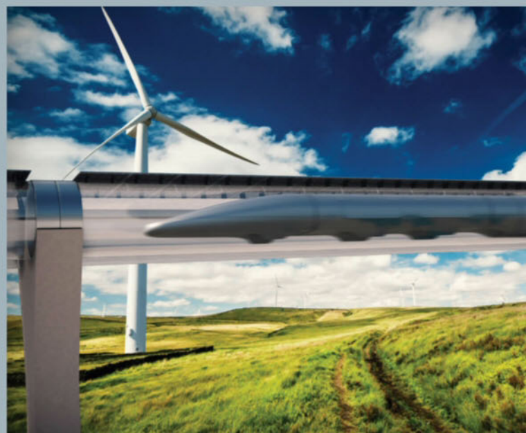
Hyperloop vacuum tubes could be raised on pylons, allowing them to be built over existing roads and minimising their footprint in other areas
